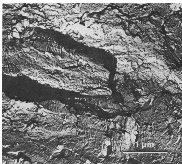
Figure 16 Transmission electron micrograph of a second-stage replica of a fracture surface of nylon-12 annealed at 260°C and 4.9 kbar for 70 h
